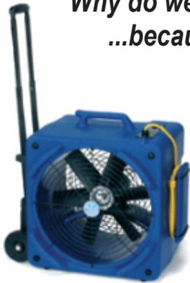
Using downdraft technology, the NEW Miniveyor Air VAF-FFD downdraft floor dryer is capable of drying an entire room in minutes. The powerful 6 blade precision fan blade draws down warmer, drier air from the top of the room and blows it across the entire floor. The powerful vane axial fan, driven by a 1/4HP 2-Speed motor, allows 360° directed airflow, and one FFD blower can dry a typical office or room in as little as 15 minutes.
